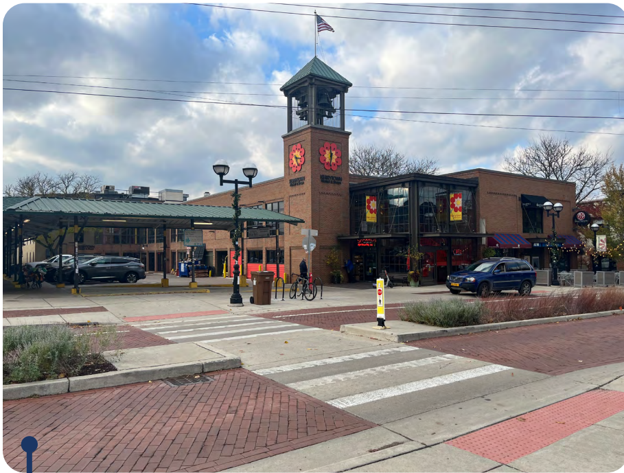
This pedestrian refuge island in the Kerrytown District of Ann Arbor allows pedestrians to focus on one direction of traffic at a time and to wait in the center if needed.
