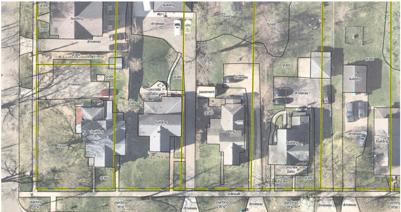
Figure 9. Example GIS-based impervious area analysis. Parcel boundaries and land-cover data are commonly used to estimate impervious area and support stormwater utility rate development and billing analysis.
